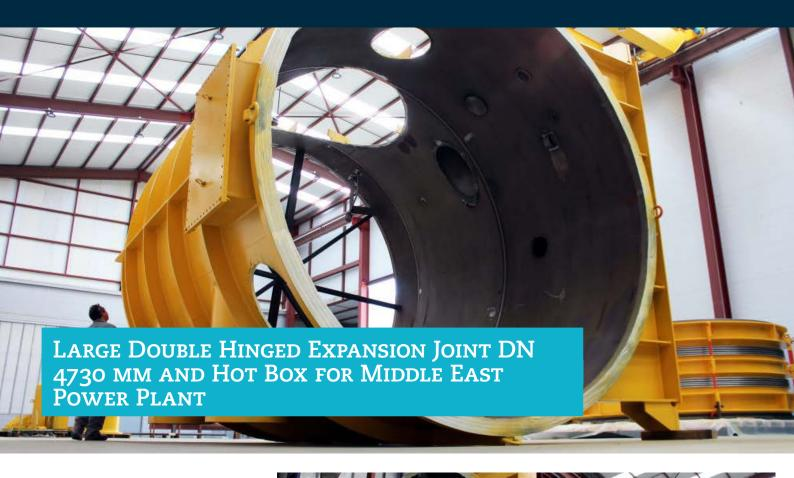
MACOGA has completed the design, manufacturing and testing of a large size MWY DN 4730 mm (186") Double Hinged Expansion Joint plus a Hot Box Duct with nozzles for a gas-fueled plant in the Middle East.
