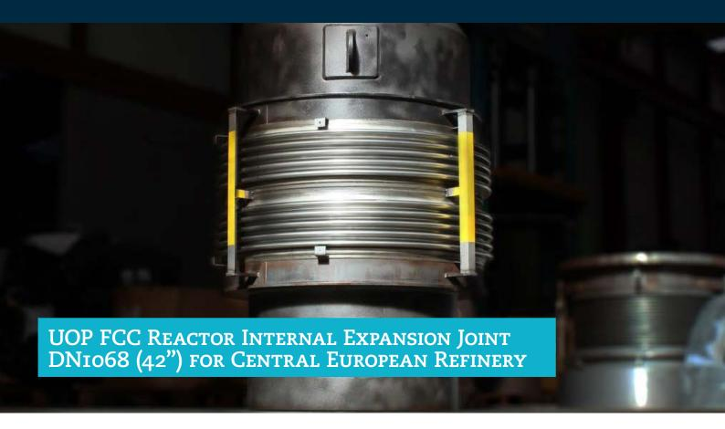
A Universal Untied FCC Reactor Internal Expansion Joint for a UOP Fluid Catalytic Cracking Process (Resid) have been successfully designed, manufactured and tested for a Central European Refinery.
