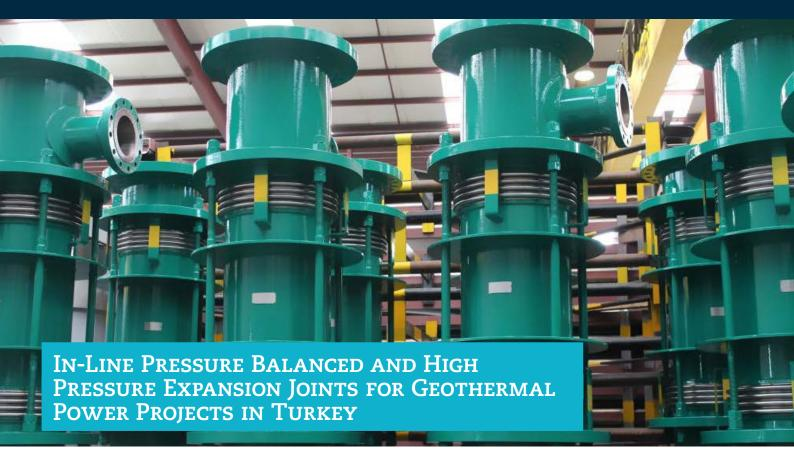
We have successfully completed the design, manufacturing and testing of 4 units In-Line Pressure Balanced and 8 units Single Axial Unrestrained Expansion Joints for a geothermal Power Project in Asia.
