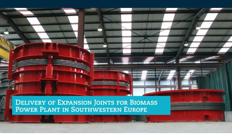
We have successfully completed the design, manufacturing, testing and shipping of 2 units Universal Tied MWL Series DN 2100 (83") and 1 unit Single Untied MFA Series DN 2800 (110") Expansion Joints for a Biomass Power Plant in Southwestern Europe.
