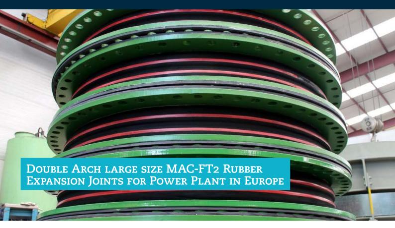
We have successfully completed the design, manufacturing and testing of 13 units MAC-FT2 Series Rubber Expansion Joints in diameters from DN1800 mm (70") up to DN2800 (110") for a new power plant in Europe.
